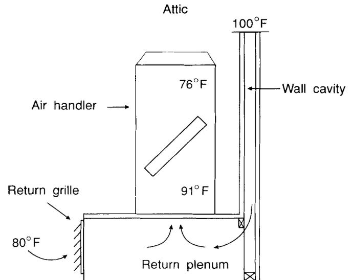
**A common problem: The air conditioner must cool 91°F air instead of 80°F air because of leaks from the attic.**
