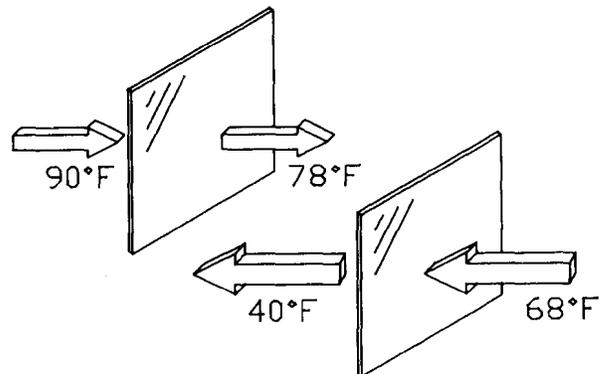
**Insulated glass is most important when temperature differences between outside and inside are high.**
