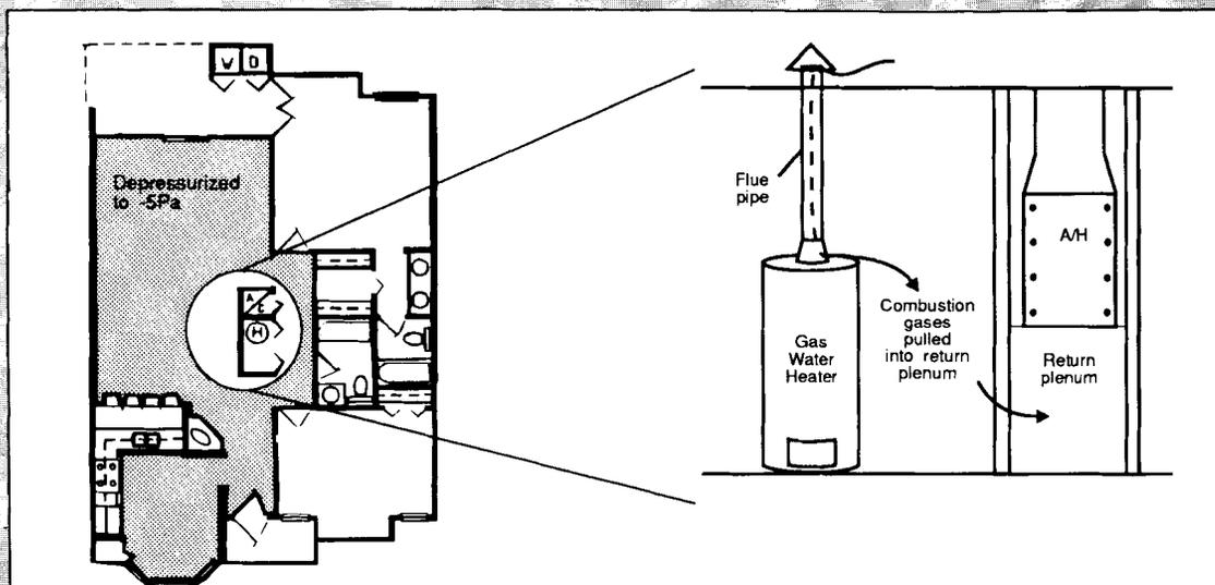
Closing bedroom and bathroom doors with the air handler on may depressurize the main body of the house, and subsequently cause backdrafting of the gas water heater.
