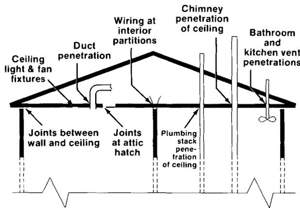
Major locations of air leakage between conditioned area and attic.
