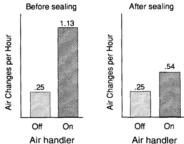
Sealing the duct system can dramatically decrease house infiltration.
