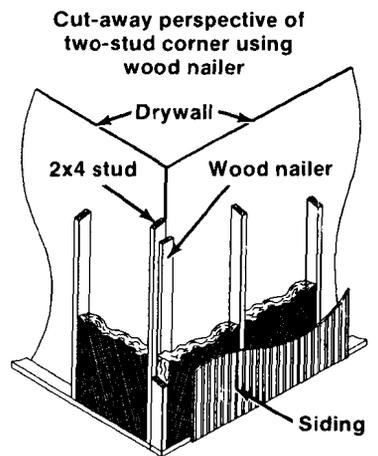
**An energy-efficient corner is constructed using two studs. Drywall can be attached using drywall clips or nailer strip.**
