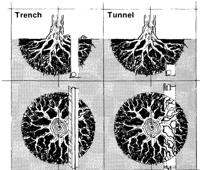
**Many roots are destroyed by trenching. Better way is to tunnel under the base of the tree.**
