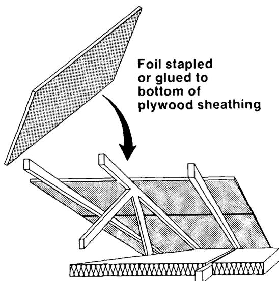
**Attaching the radiant barrier directly to the sheathing can reduce installation costs.**
