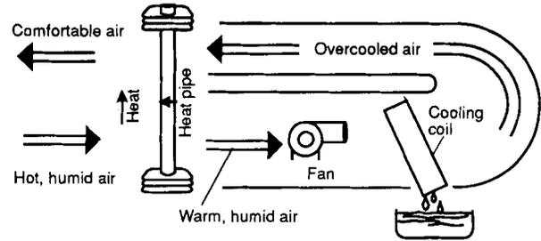
A heat pipe precools return air with overcooled supply air to provide more moisture removal.
