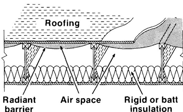
Use plywood-webbed I-beams to assure air space for ventilation and radiant barriers (if used) in cathedral roofs.
