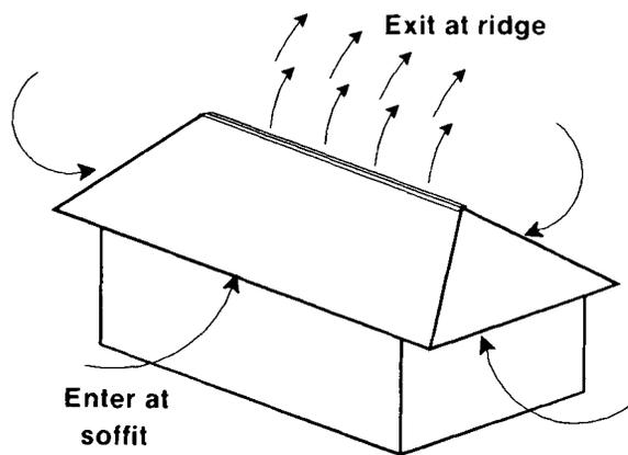
**Attic air flow is best with continuous soffit and ridge vents.**
