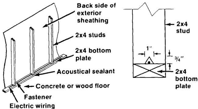
**Use notches for wiring to prevent insulation from being compressed.**
