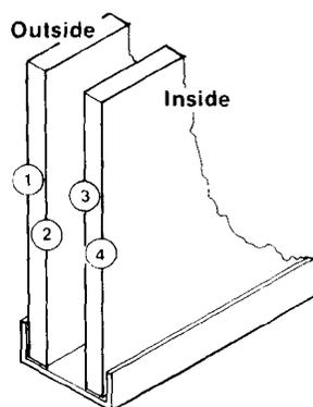
**The low-e coating in insulated units faces the airspace and absorbs heat. Having the coating on surface 2 rather than surface 3 more effectively block the sun's heat from the house.**
