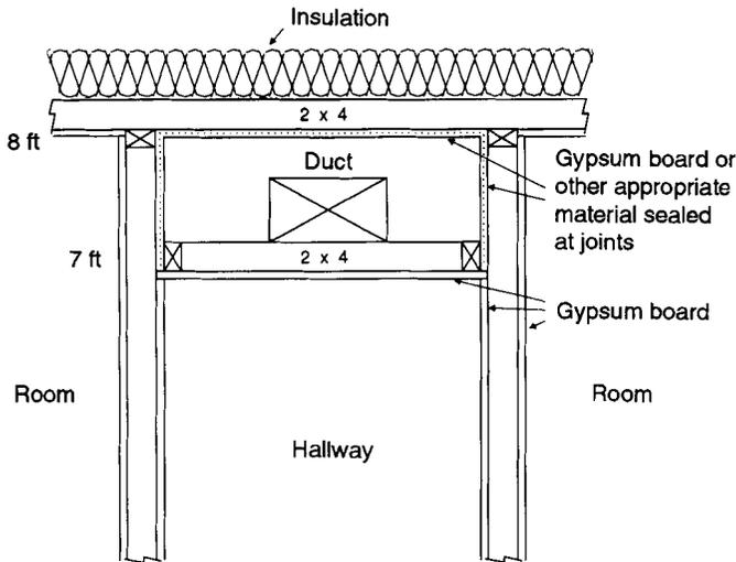
**Isolate ductwork from unconditioned space with a continuous air and heat barrier.**
