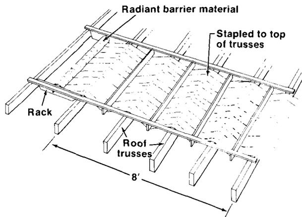
**An easily-built radiant barrier installation rack.**
