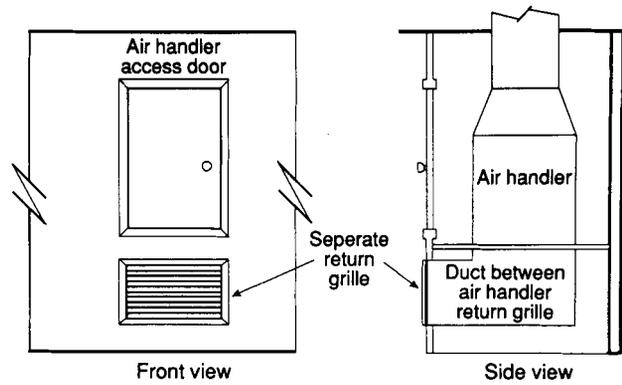
Use a solid door for air handler access and a separate sealed return duct from the air handler to a grille below.
