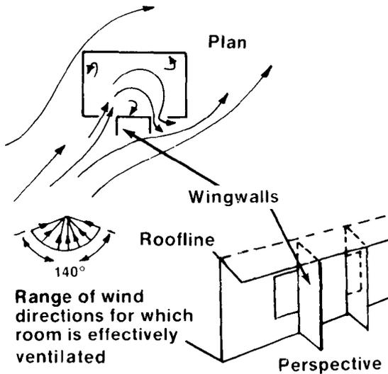
**Wingwalls create inlets and outlets for ventilation of rooms with one outside wall.**
