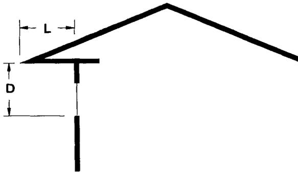
The length (L) of a south-facing overhang can be determined by knowing the sill-to-soffit distance (D).
