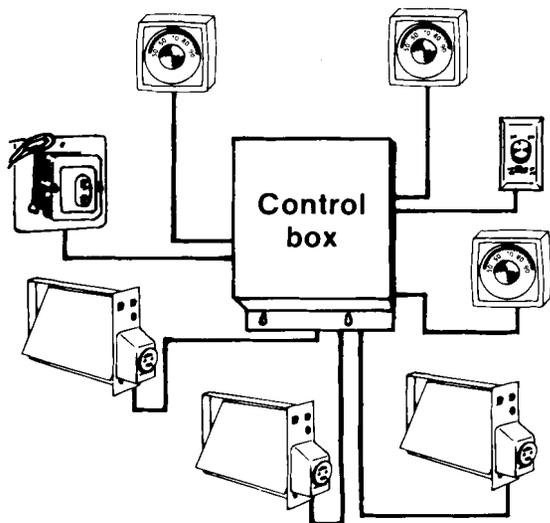
**An automatic multizone control system has a controller, plus thermostats and dampers for each zone.**
