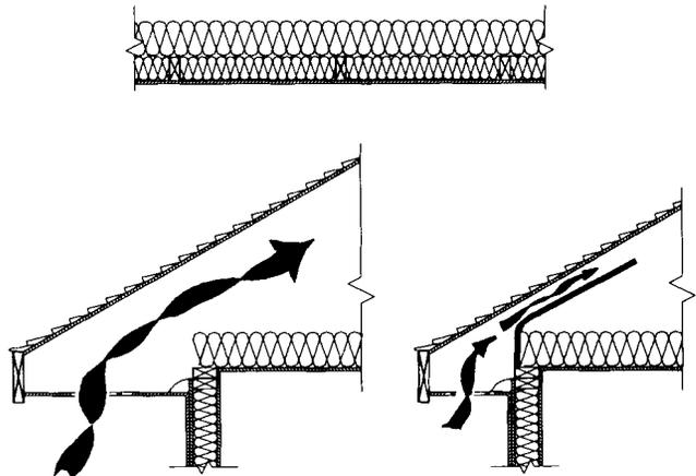
Insulation should extend over the top ceiling joints and ventilation should be provided at the eaves with extended trusses or baffles.
