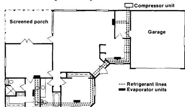
A multi-evaporator system sends refrigerant to individual room conditioning units, eliminating ductwork.
