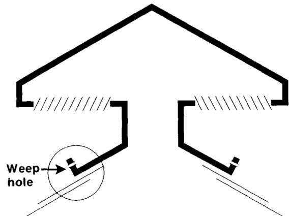
A ridge vent of this type is effective in resisting wind-driven water from backing up into openings. Weep hole is present in end flange.
