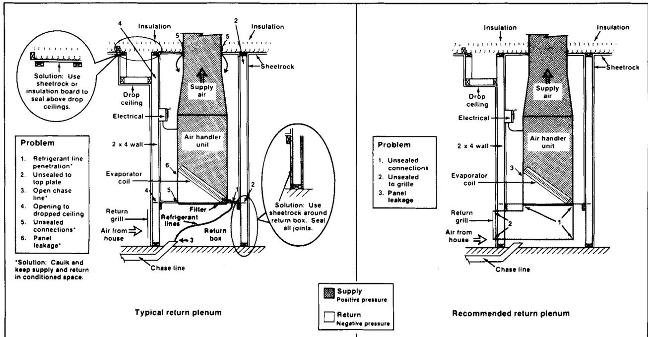
Typical leakage points in air handler systems. (Based on illustration by Natural Florida Retrofit, Inc.)
