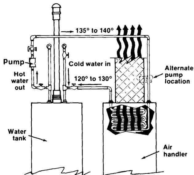
**Forced-air hydronic systems use hot water to supply heat.**
