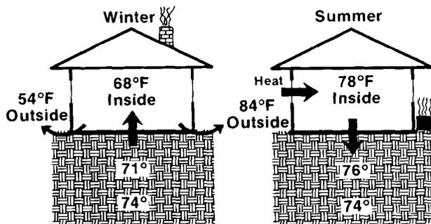
**In winter, heat flows in from the earth and out through the slab perimeter. In spring and summer, the ground helps remove heat.**
